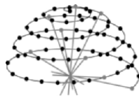
Fig. 1 The center of mass is established from the first interleave of a 3D PR trajectory.
